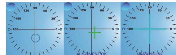
Figure6.3 Move the lens to make it alignment the target
