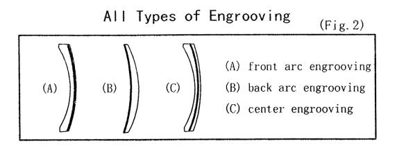
A. Center Groove – Used for plus lenses or thin lenses with uniform edge thickness.
