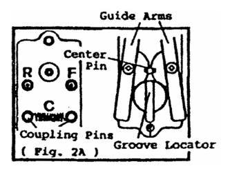
B. Front Curve Groove – Used for high minus lenses with high cylinder curves.
