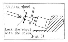
**CAUTION**: The cutter wheel must be replaced correctly (Fig. 3) so that it fits into the slot of the lens acceptor (Fig. 1)
